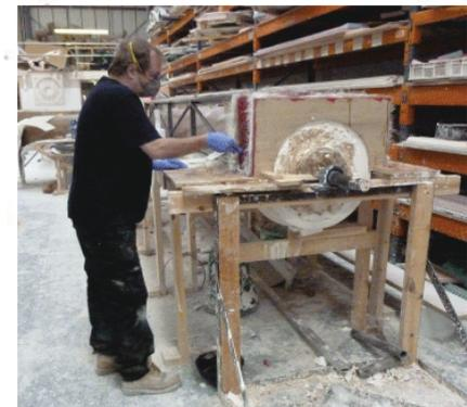
Pictured above is the manufacture of a fluted column master. The columns are to be made in Scagliola. Mike Berry a Scagliola craftsman is pictured making the fibreglass mould casing.
